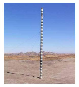
Figure 36: Multivertical dust sampler
