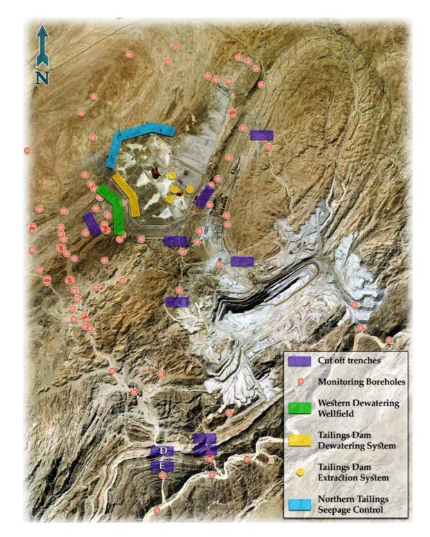
Figure 29: Location of monitoring boreholes at the Rössing mine site Figure 30: Delineation of the seepage plume surrounding the tailings storage facility (yellow line). Affected bores close to the seepage front are indicated with red circles; unaffected bores with green circles.
