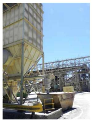
Figure 20: Fine crushing dust collection system
