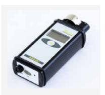
Figure 24: MyRIAM instrument The calculated dose depends on the weighted dose conversion coefficient (as discussed in Section 4.5.2.1) which has to be entered into the instrument software prior to monitoring. Three different dose conversion coefficients are entered according to the type of dust inhaled (see Table 7 above). It should be noted that the beta dust conversion coefficients are about two orders of magnitude smaller than those for alpha particles, and hence these are disregarded.
