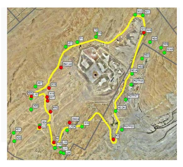
Borehole monitoring at Rössing Uranium is used to produce a map depicting the seepage plume around the TSF. An example of the plume is shown in Figure 30.
