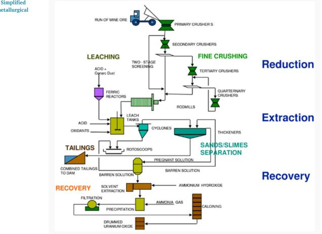
**Figure 4: Simplified** flow of metallurgical process
